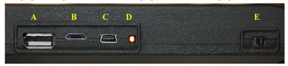
**E. On/Off** – **Fast Charge:** Turns meter on for use. Turn off to conserve battery or for faster charging.
