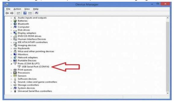
**22A. Set Up Procedure:** Allow the computer to assign a comport and install FTDI drivers, as needed. Device drivers are located in C, Program Files, International Light Technologies, ILTdevice Software Suite, FTDI folder. To install drivers double click driver CDM.....exe
